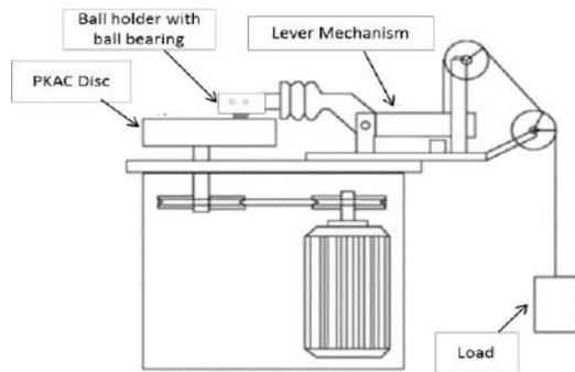
Fig. 2 Schematic diagram of ball on disc tribometer
