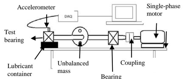
Fig. 1 The schematic layout of the measurement system
