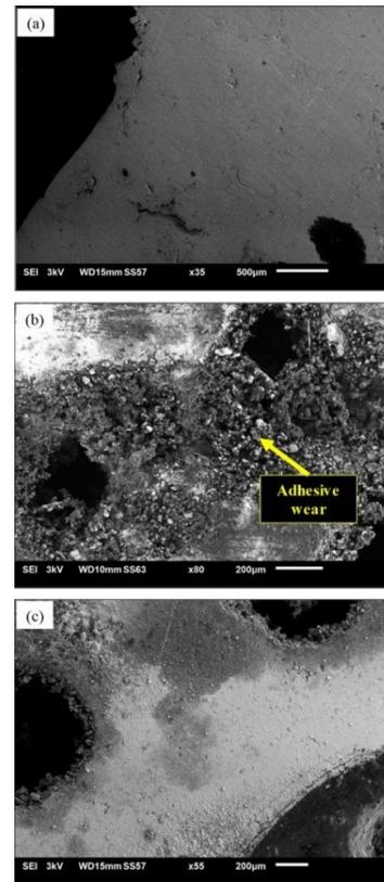
Figure 2 SEM micrograph of worn surfaces of (a) non-textured surface, (b) 500 $\mu\text{m}$  and (c) 1000 $\mu\text{m}$  in diameter dimples.
