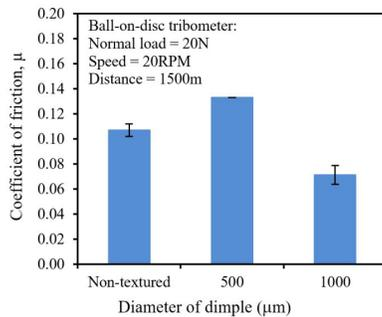
Figure 1 Effect of dimple size on COF of PKAC-E.
